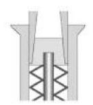
As shown in upper figure, leakage of solution and infection may occur due to the breakage of the injection port of syringe with an internal diameter of  $\bigcirc$  mm or less
