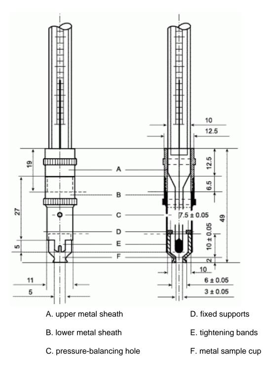
Figure 1. Apparatus for the determination of drop point
