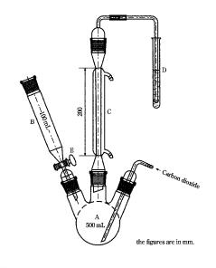
A: Boiling flask (500 mL) B: Funnel (100 mL) C: Condenser
