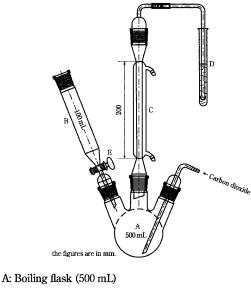
A: Boiling flask (500 mL) B: Funnel (100 mL) C: Condenser D: Test-tube E: Tap
