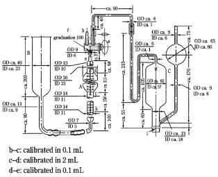
c-d: calibrated in 2 mL d-e: calibrated in 0.1 mL e-f: calibrated in 0.1 mL The graduations are marked with red line. b-f: =100 mL
