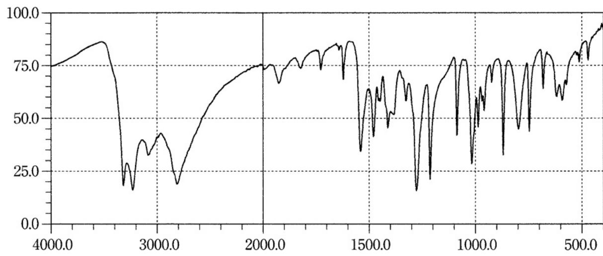
Preparation of sample: Potassium chloride disk method
