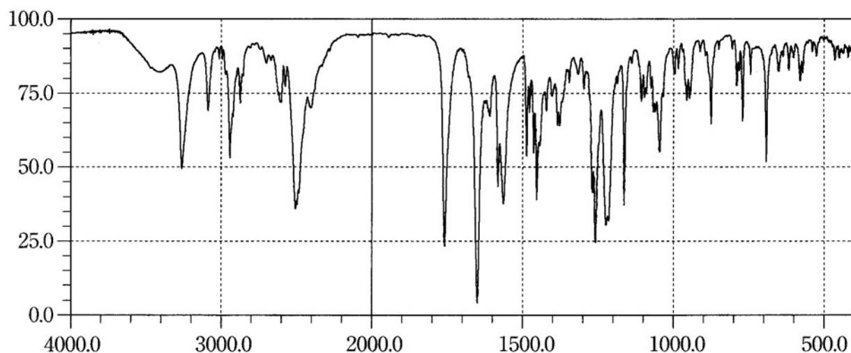
Preparation of sample: Potassium chloride disk method
