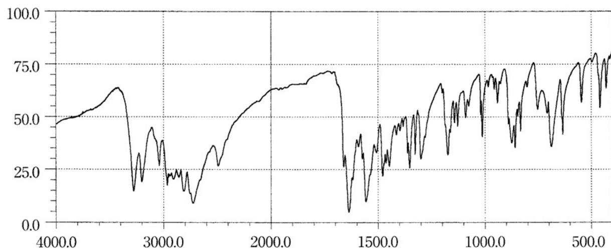
Preparation of sample: Potassium chloride disk method
