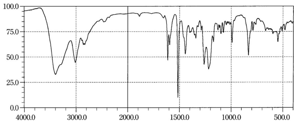
Preparation of sample: Potassium chloride disk method
