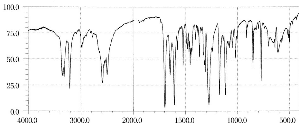
Preparation of sample: Potassium chloride disk method
