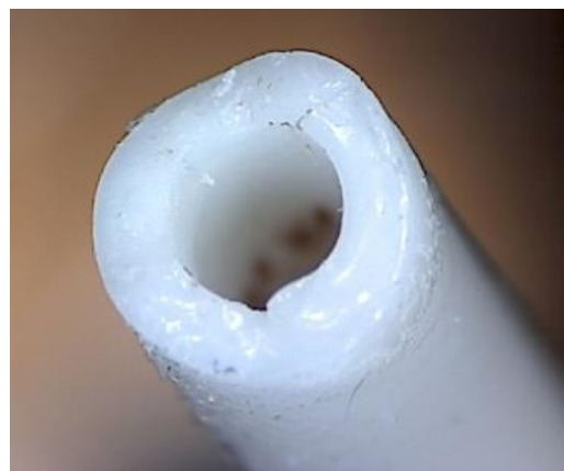
Example of a fractured catheter
