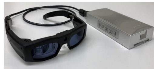
Size of control box: 160 mm × 80 mm × 31 mm
