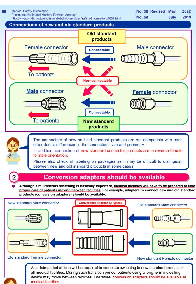
As shown in the upper figure, two different types of conversion adapters exist and caution should be taken. Please check with the MAH, etc. for the handling of conversion adapters.
