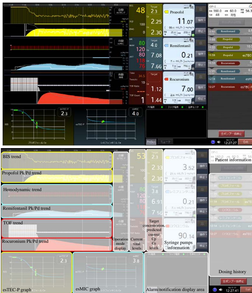
Figure 2. Information that Robotic Anesthesia System displays on general-purpose computer (top) and description of the screen (bottom)
