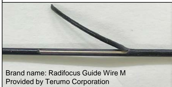
A guidewire with a peeled-off coating
